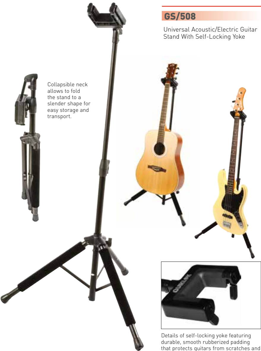
When the guitar is placed into the stand yoke, the instrument's weight will automatically drive the lateral safety barriers to turn down and lock the guitar neck securely in place, preventing the instrument from accidentally falling off the stand.
