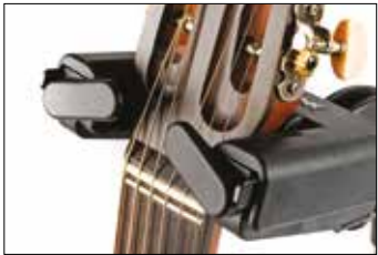
When the guitar is placed into the stand yoke, the instrument's weight will automatically drive the lateral safety barriers to turn down and lock the guitar neck securely in place, preventing the instrument from accidentally falling off the stand.
